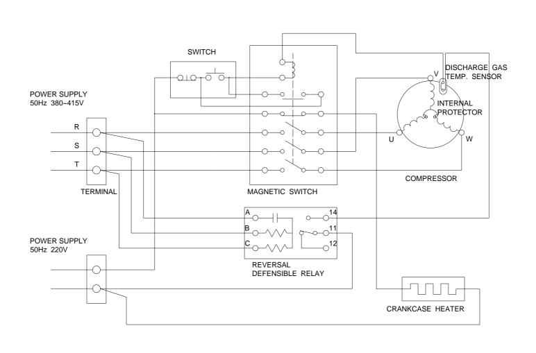
Part Code E-0910-DSC Name Wiring Diagram
