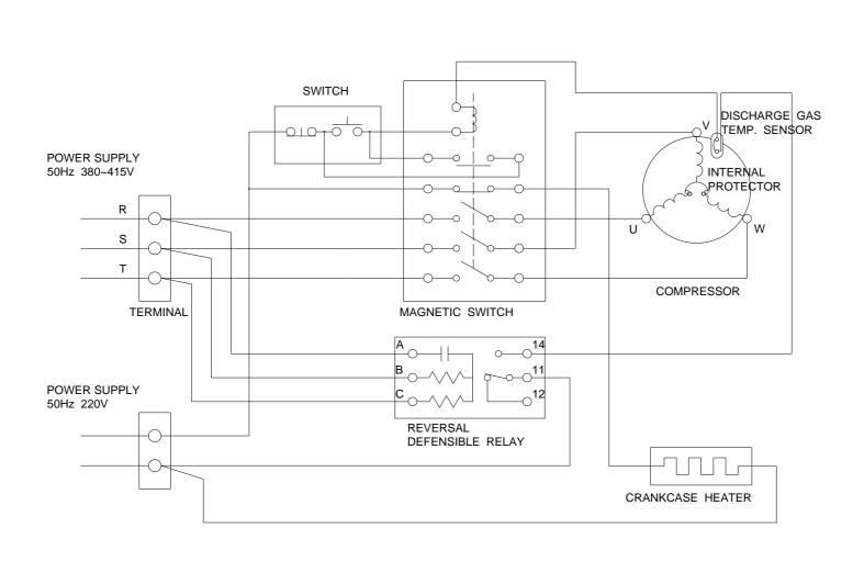
Part Code E-0910-DSC Name Wiring Diagram
