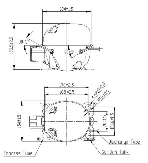
Caution:Suction tube and process tube can not be exchanged
