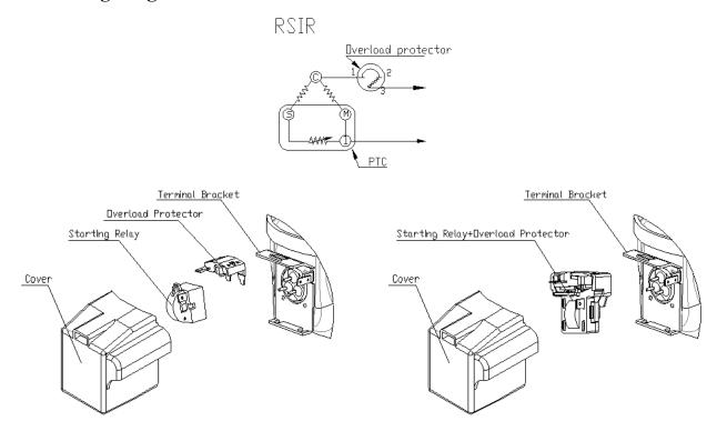
Note: Each of the starting relay, the overload protector and the cover is separately provided by our company.
